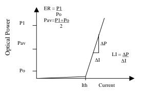
Figure 1. Laser Transfer Function
